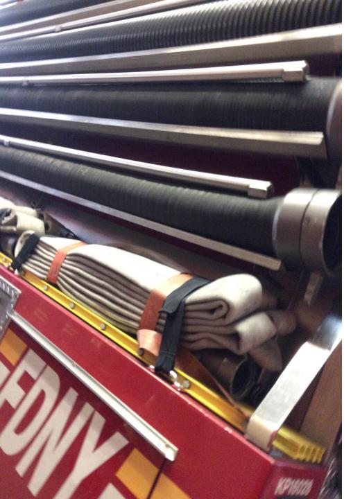
Did you ever notice these hoses? They are super long and are very useful! Some hoses attach to holes on the side of the truck) and they connect the water (from the fire hydrant) into the truck and then they need to get another hose to connect into the water in the truck. Sort of confusing right?
