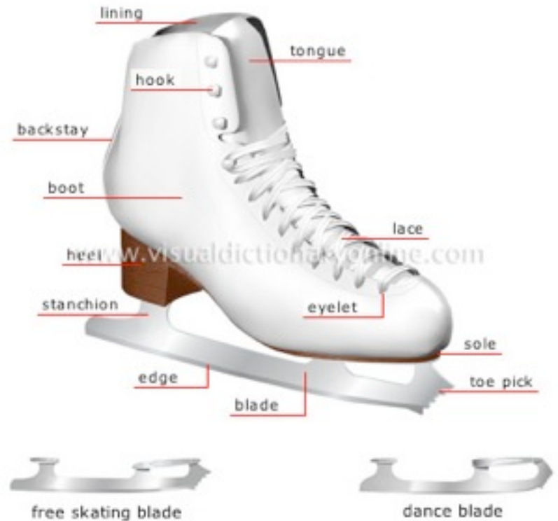
DIAGRAM OF A FIGURE SKATE
